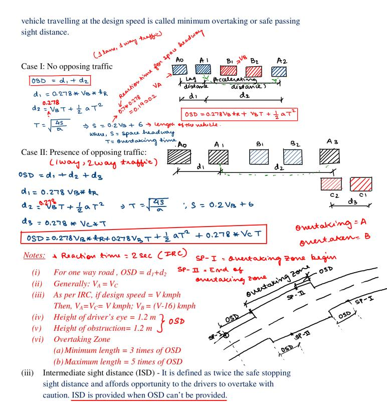
a. On a two way traffic road, the speed of overtaking and overtaken rehides are 100 kmph & 50 kmph respectively. If the average acceleration is 1 m/sec<sup>2</sup>, determine the OSD.
